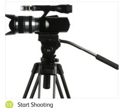
If you do not need to pan or tilt during your shot, keep the pan and tilt knobs locked.
