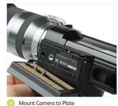
Attach the mounting plate to your camera. Be certain that the retractable alignment pin sets into its pocket on the camera. Screw the threaded stud on the plate into the bottom of the camera, making certain that the plate is placed at the camera's center of gravity.
